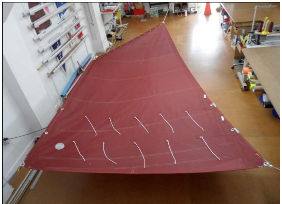
Standing lug sail under construction
