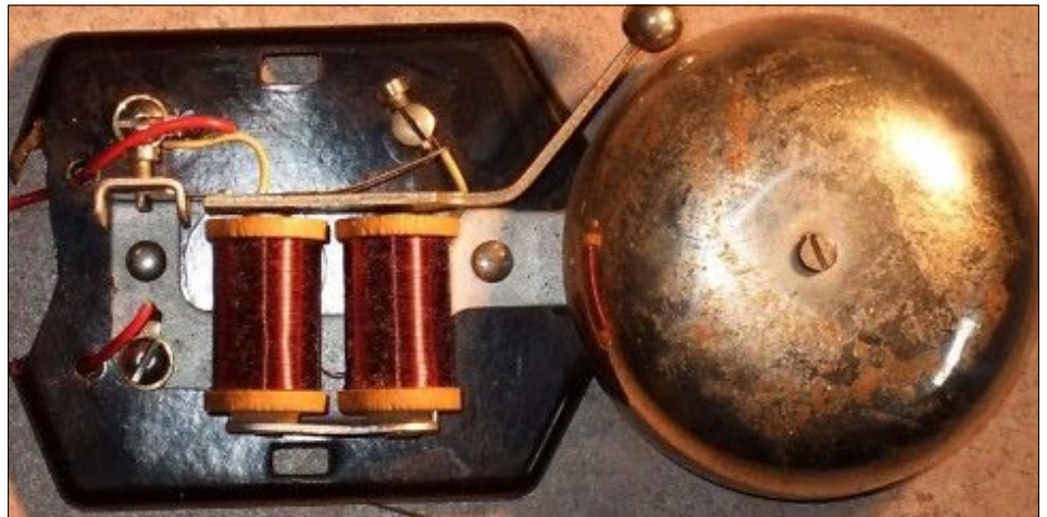
An old fire alarm bell, with new wiring but without its weatherproof cover.
