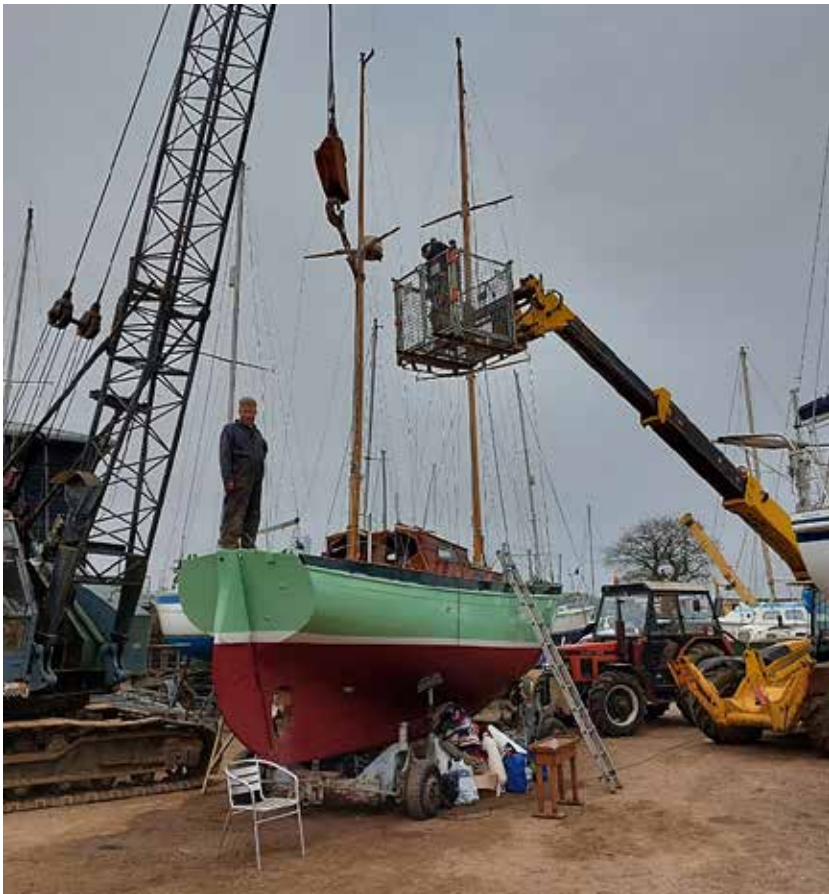
Masts – stripped back to bare and sanded fair – are lowered into place
